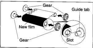
Insert the four gears into the new film cores so that the guide tabs of each gear fits into the slots of the film core.
